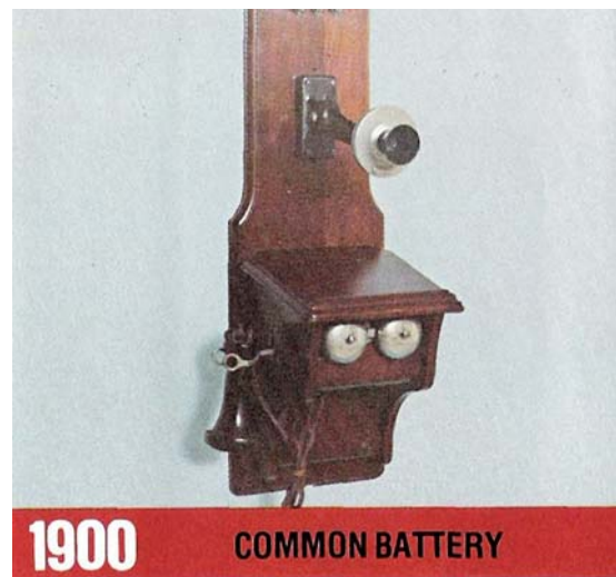
Improving telephone service is a constant goal. The earliest sets were voice-powered. Next came the wet battery, which occasionally leaked on the rug; then the dry battery. This model, a major advance, received its power from the telephone exchange, hence its name.
